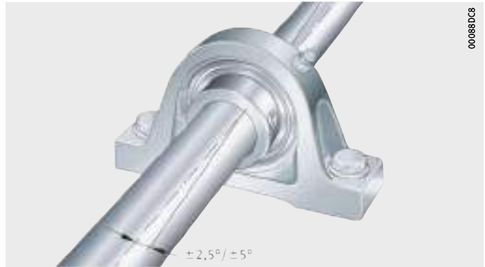
Figure 1 Compensation of static shaft misalignment
