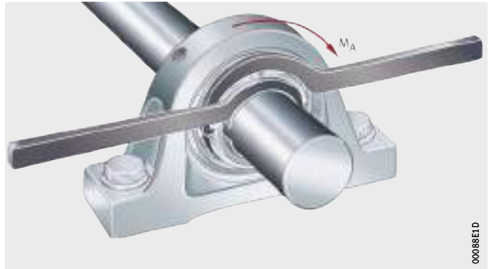
Figure 6 Tightening of locknut
