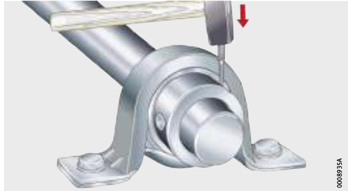
Figure 13 Tensioning the eccentric locking collar
