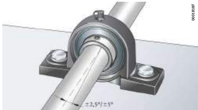
Figure 3 Compensation of static shaft misalignment
